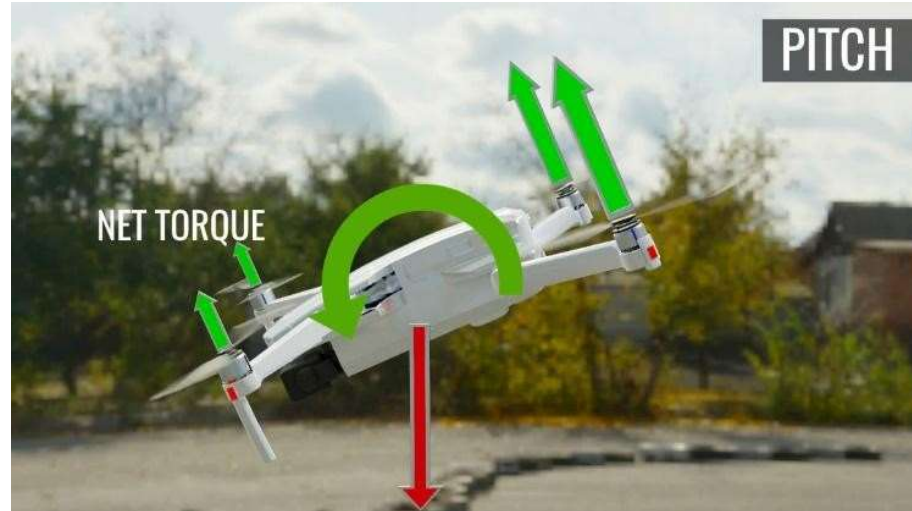
Figure 3.4: Forces acting on a drone during pitch motion.
