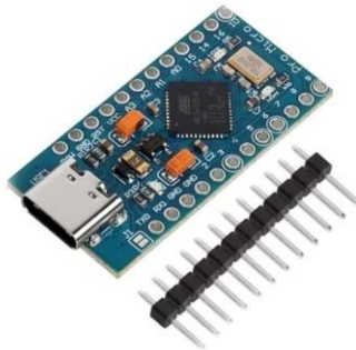
Figure 2 Arduino Micro board used in the device.
